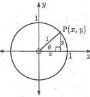
$\theta$  is positive when measured in an anticlockwise direction from the positive x-axis.
